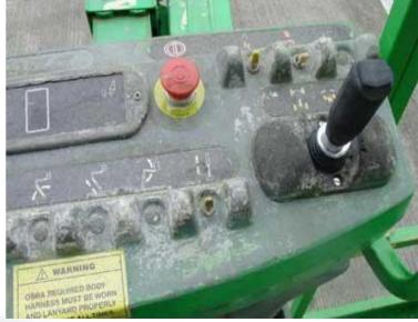
Before moving an aerial lift for travel, the boom(s) must be properly cradled and outriggers must be in stowed position.
