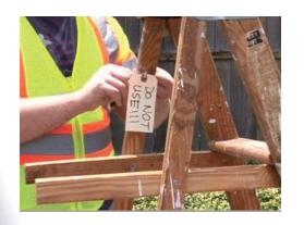
Ladders that are damaged or defective can be very dangerous. OSHA requires all portable ladders found to have structural defects immediately be marked or tagged "DO NOT USE" and taken out of use until repaired.
