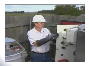
2. Machine or equipment shut down. The machine will then be shut down according to the procedures required by the manufacturer. An orderly shut down must be used to avoid increased hazards to employees as a result of incorrect shut down.
